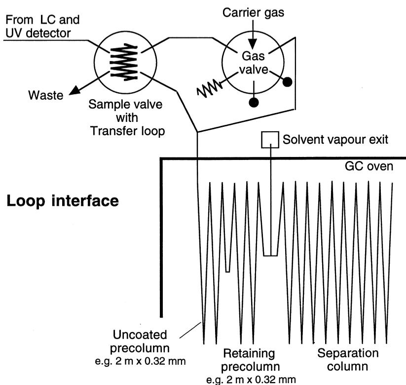
Fig. 1. Loop type interface for LC–GC transfer involving concurrent eluent evaporation. Discharge of the eluent vapours by overflow.
