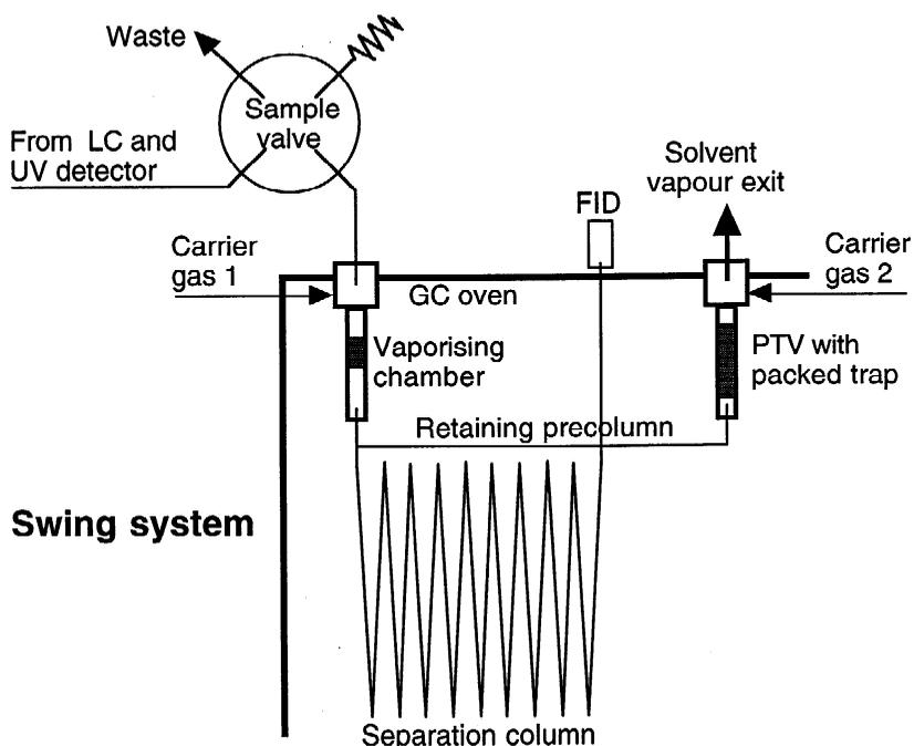
Fig. 7. Swing system for better retention of the volatile solutes.
