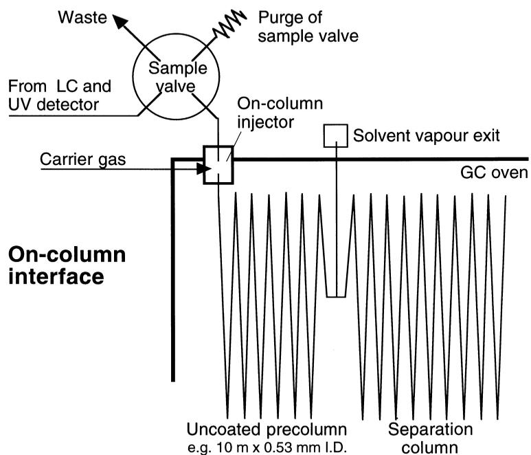
Fig. 2. On-column interface, mostly used for the transfer of wetting liquids by the retention gap technique (partially concurrent evaporation).
