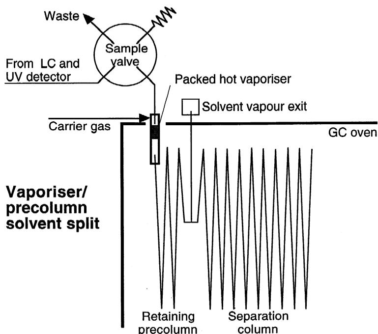
Fig. 6. Vaporiser/precolumn solvent split interface. When used for non-wetting mobile phases, vapours are discharged through a retaining precolumn.
