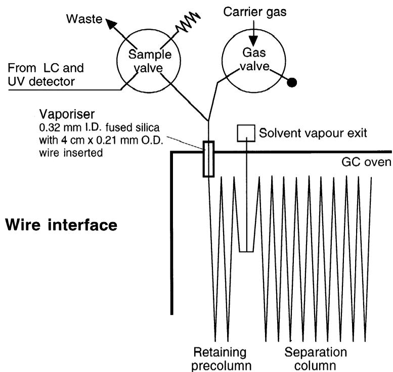
Fig. 3. Wire interface for concurrent evaporation of organic eluents.
