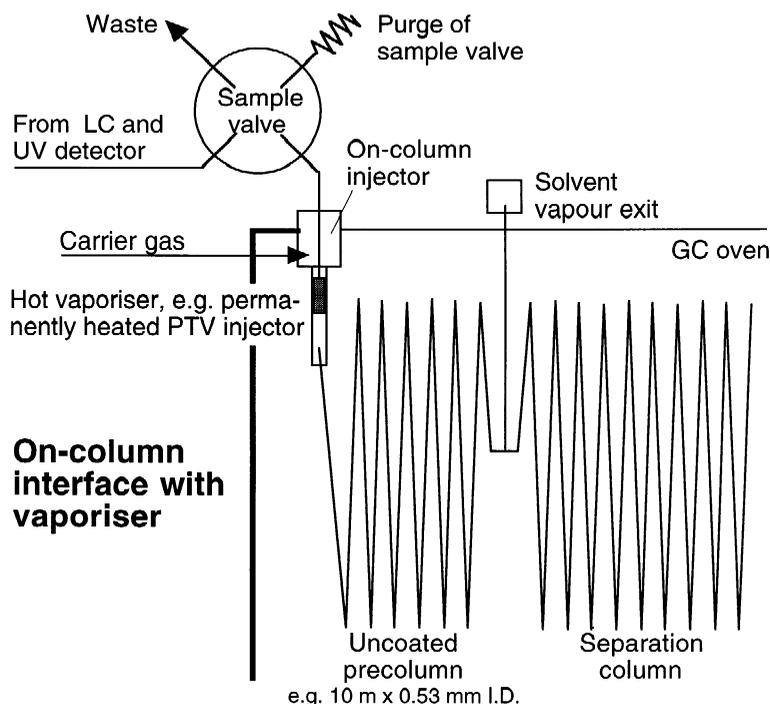
Fig. 5. On-column interface with a vaporising chamber above the uncoated precolumn acting as a filter retaining non-evaporating by-products, here shown as a PTV injector mounted to the bottom of an on-column injector (system Fisons/CE Instruments).
