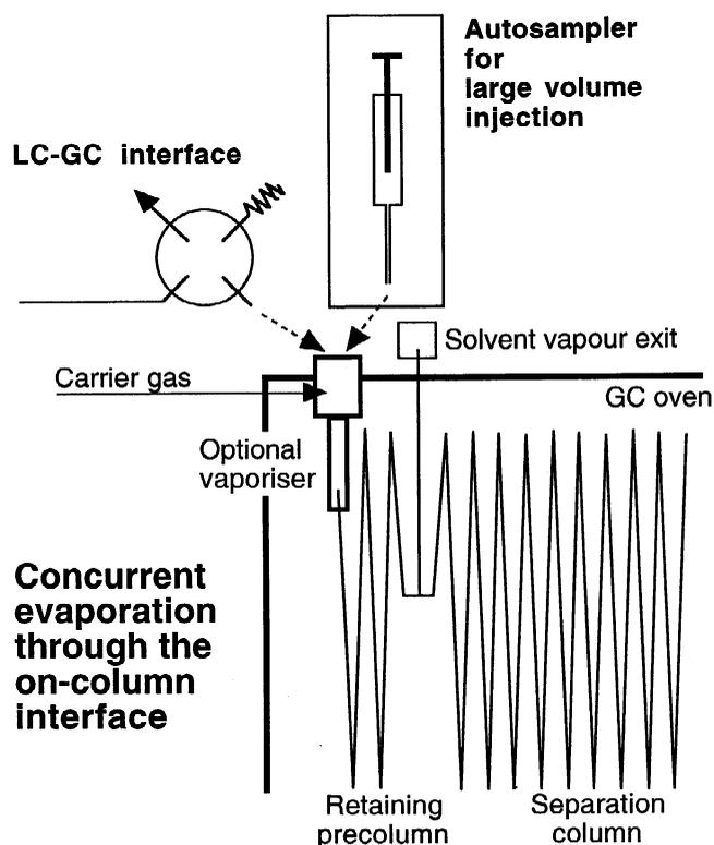
Fig. 9. Concurrent evaporation with the on-column interface for large volume injection as well as on-line LC–GC.
